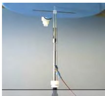
Photograph of the dipole Antenna
