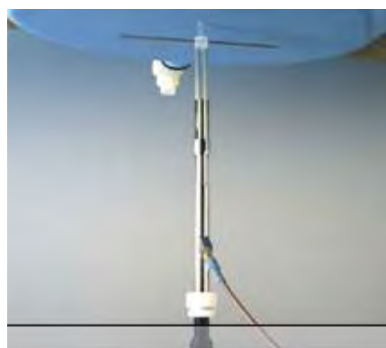
Photograph of the dipole Antenna
