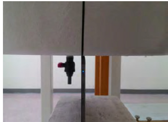
Fig.3 EUT Top side to flat phantom
