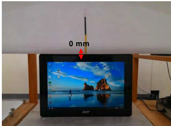
Fig.3 EUT Top side to flat phantom
