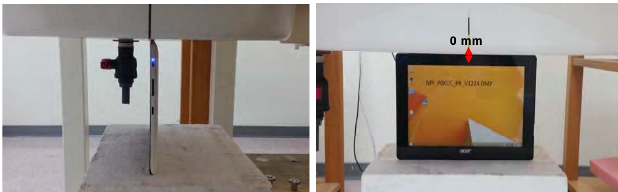
Fig.4 EUT Top side to flat phantom
