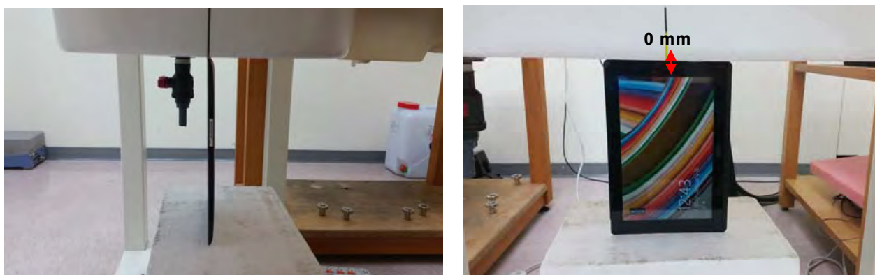
Fig.5 EUT Right side to flat phantom
