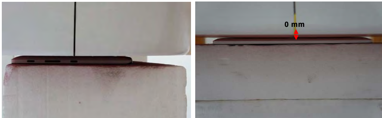
Fig.3 EUT Lap-held mode to flat phantom
