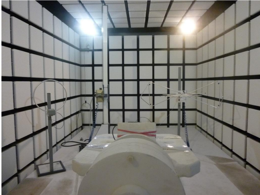
Photo 3: EUT with PCB antenna at the anechoic chamber
