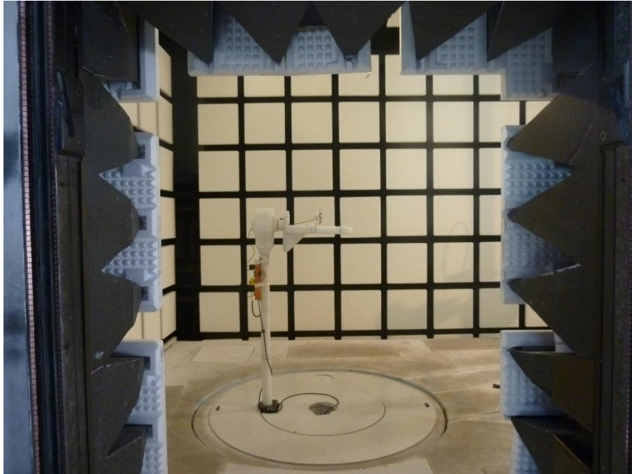
Photo 1: EUT with PCB antenna at the anechoic chamber
