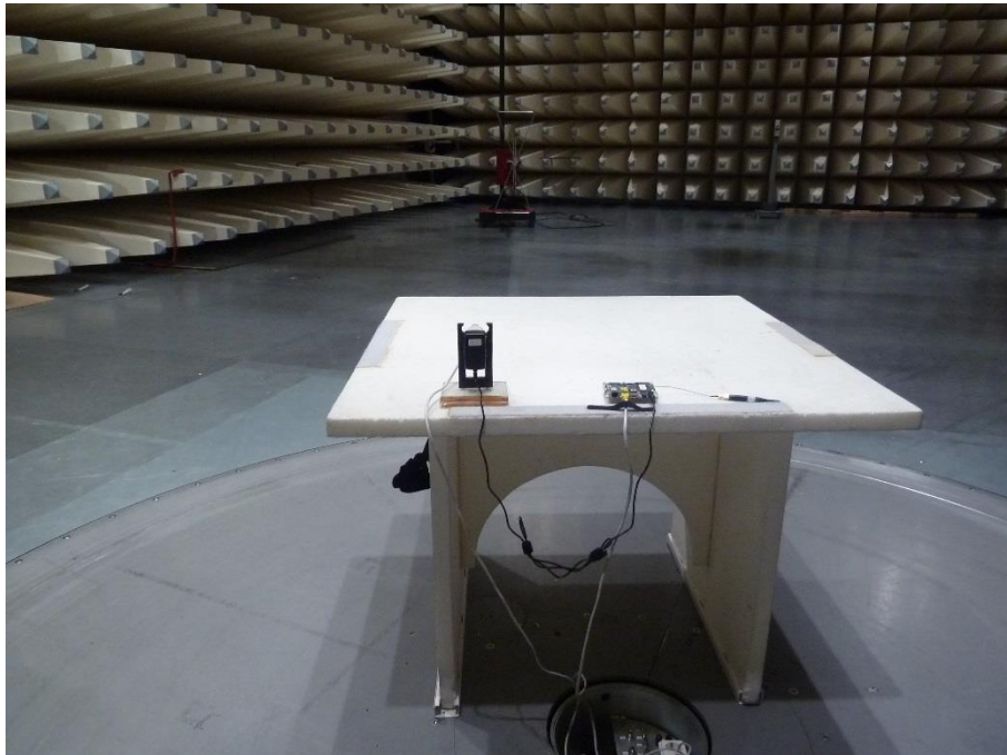
Photo 15: EUT with dipole antenna at the anechoic chamber
