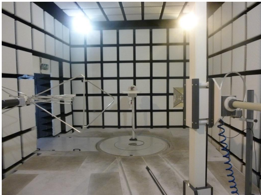
Photo 6: EUT with PCB antenna at the anechoic chamber
