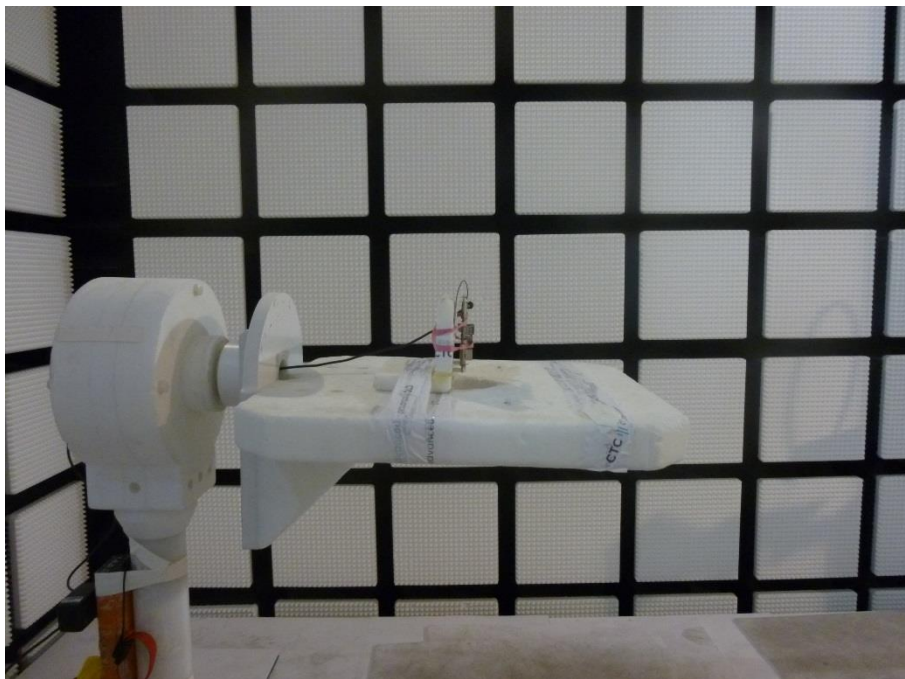
Photo 2: EUT with PCB antenna at the anechoic chamber
