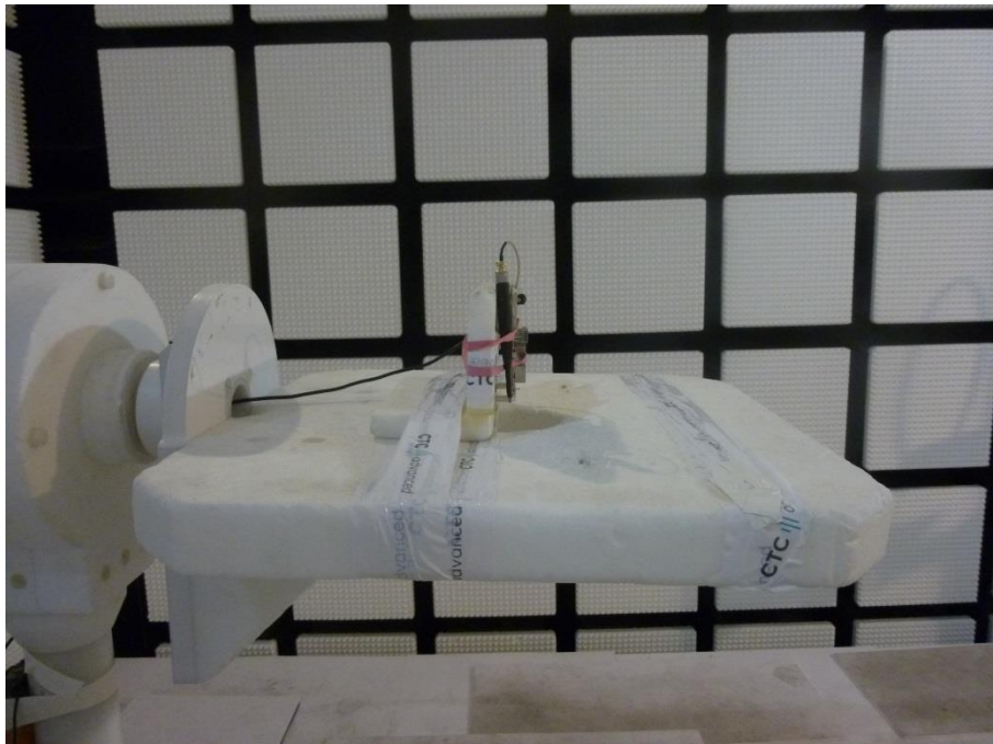
Photo 8: EUT with dipole antenna at the anechoic chamber
