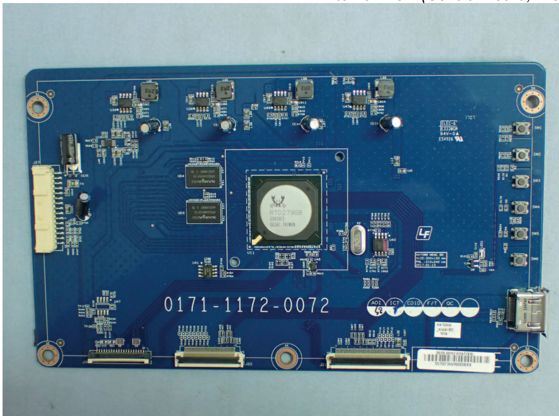
Figure 25 Internal View (Control Board, Front View)
