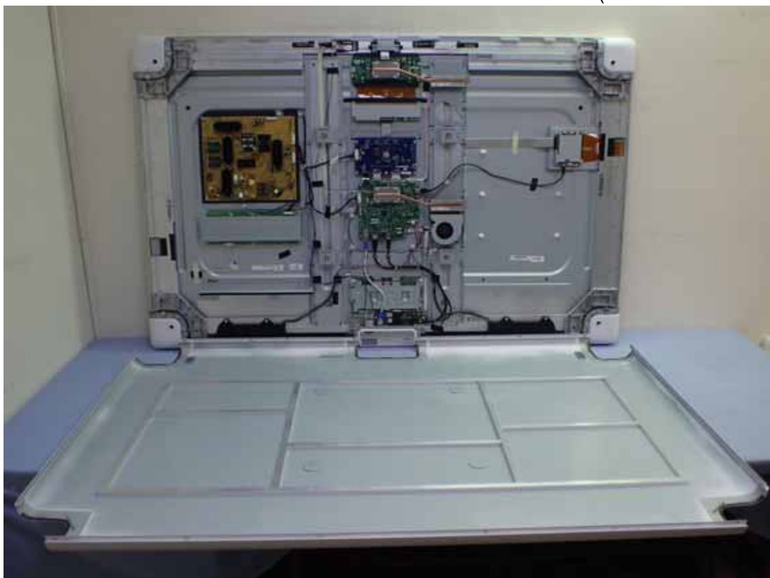
Figure 4 Internal View (Removed Back Cover)
