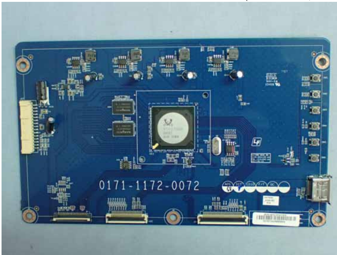
Figure 17 Internal View (Control Board, Front View)
