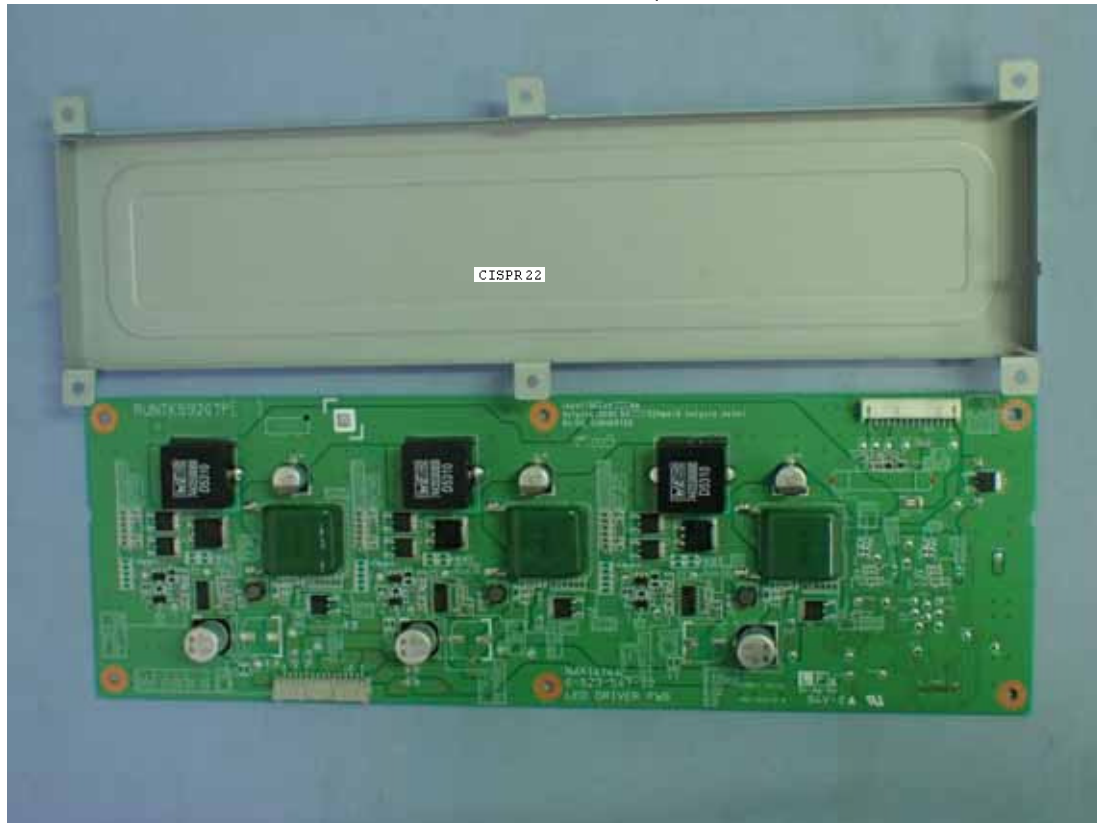
Internal View (DC/DC Converter Board, Front View)
