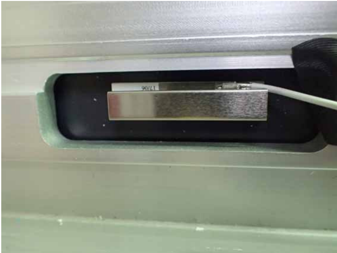
Figure 7 Internal View (Antenna View)
