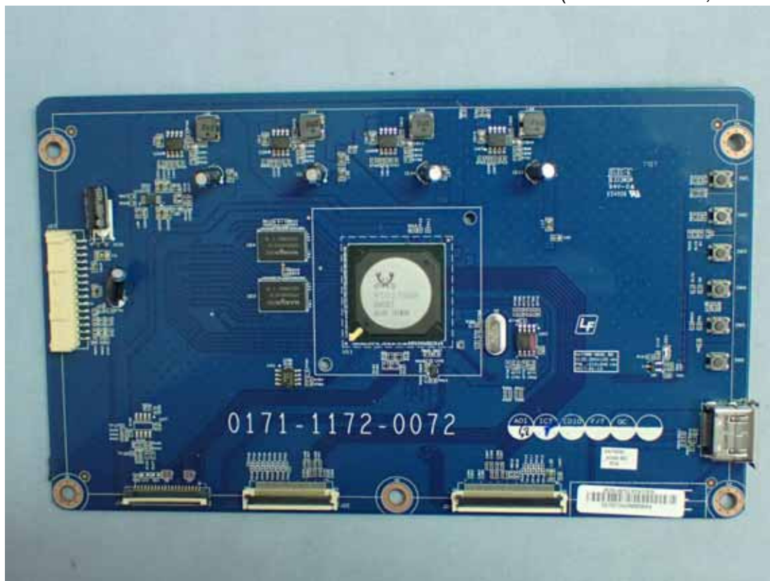
Figure 17 Internal View (Control Board, Front View)
