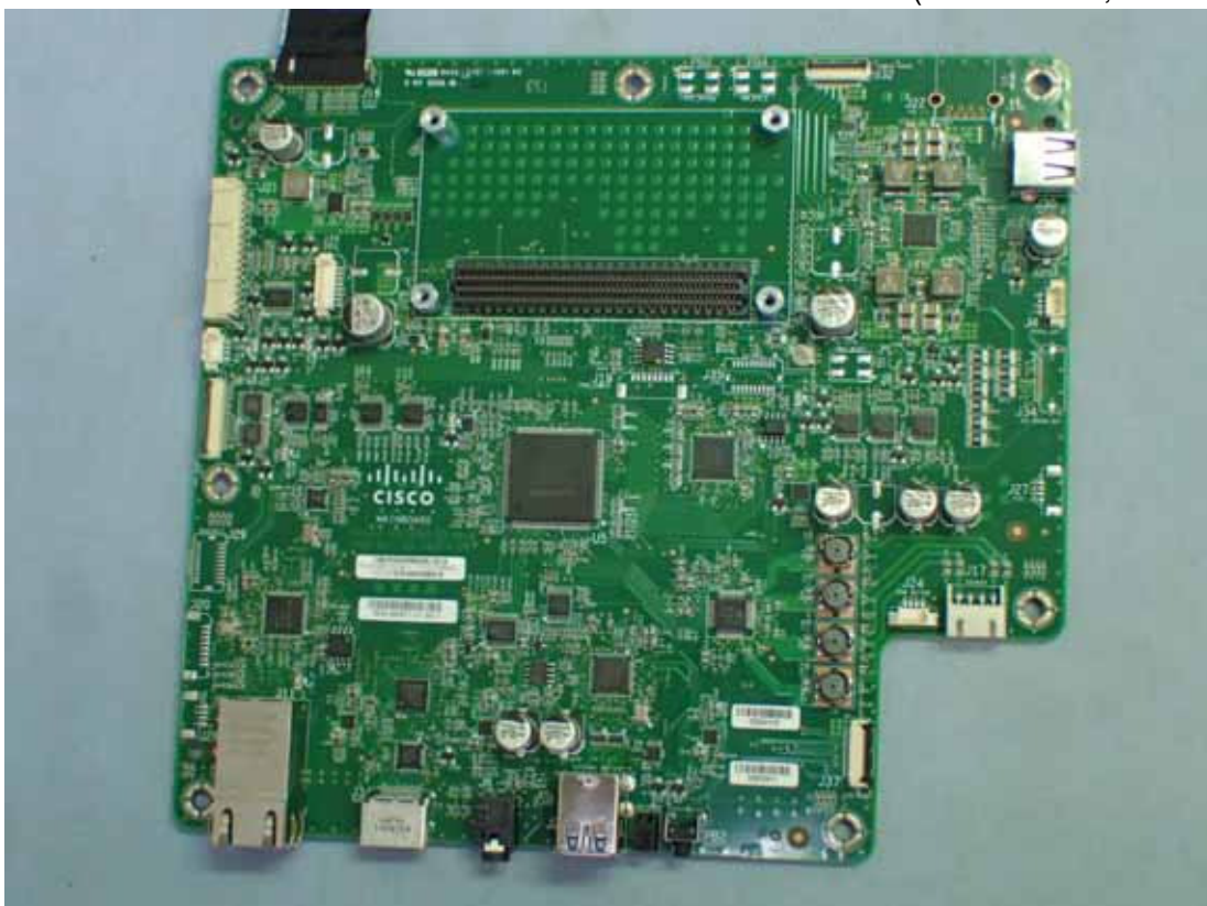
Figure 24 Internal View (Main Board, Front View)
