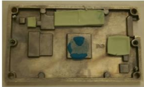
Heat Sink Internal View
