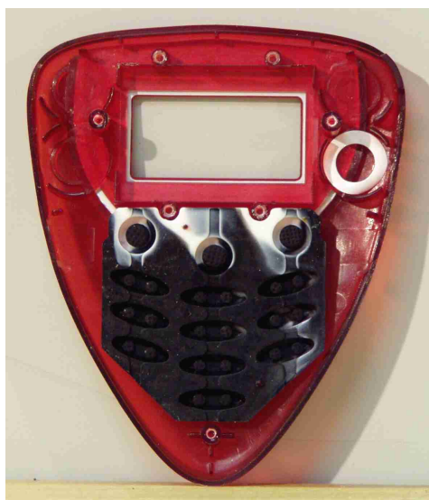
Inside view, PCB removed.
