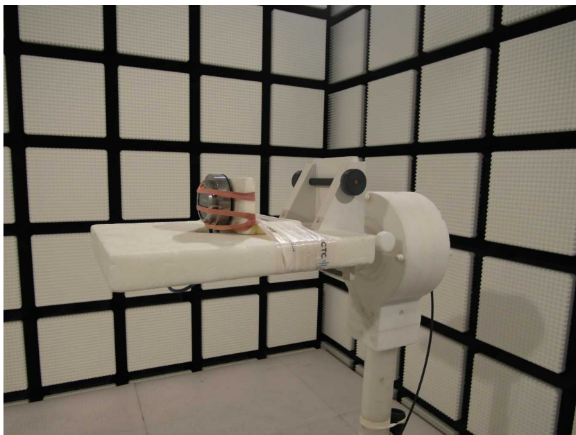
EUT at the anechoic chamber
