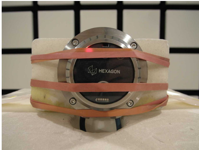
EUT at the anechoic chamber
