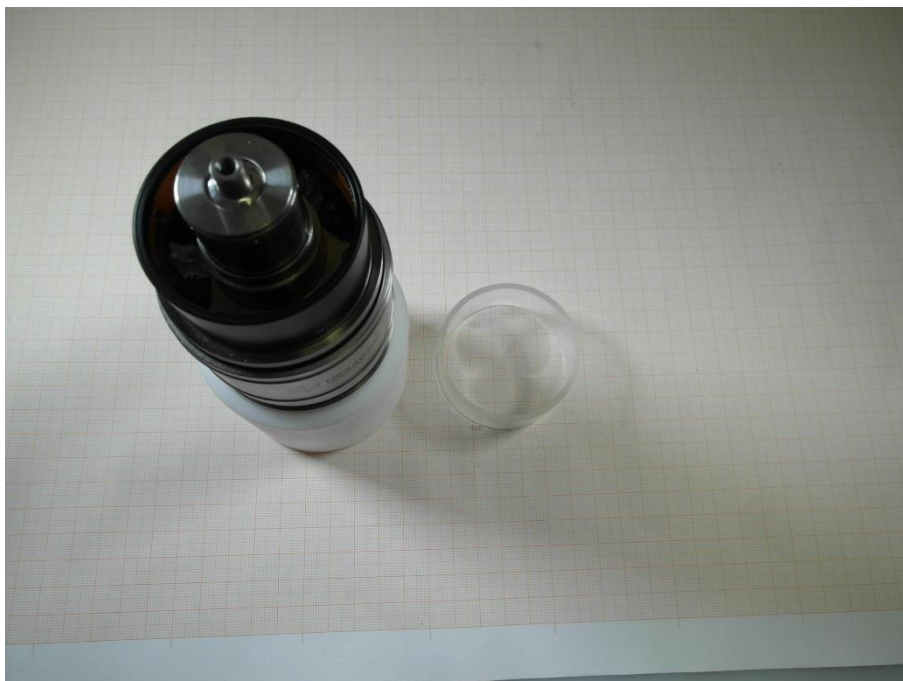
Photo 4: antenna shelter (glas)
