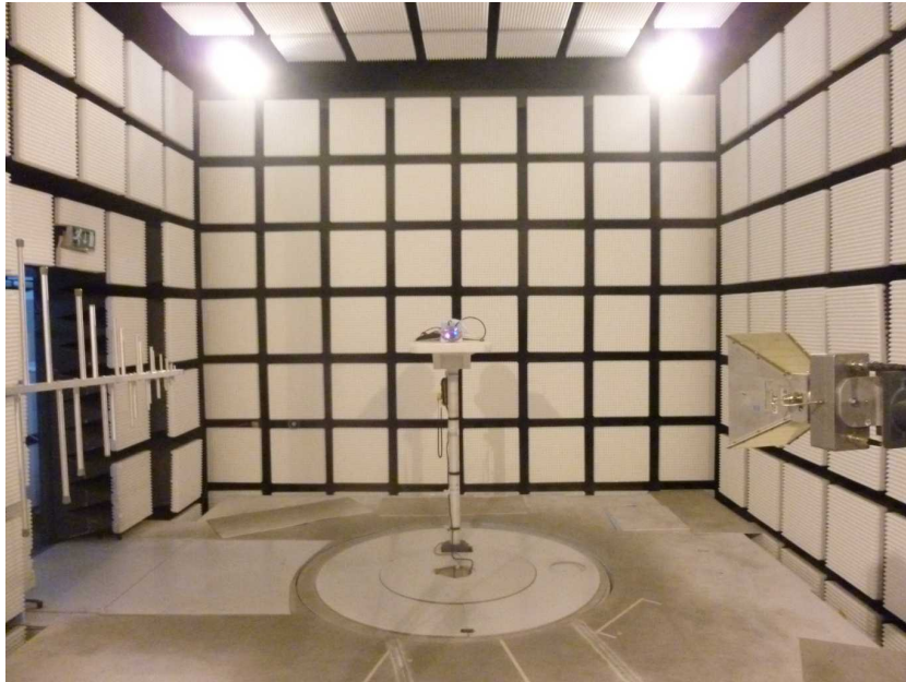
Photo 5: EUT at the anechoic chamber
