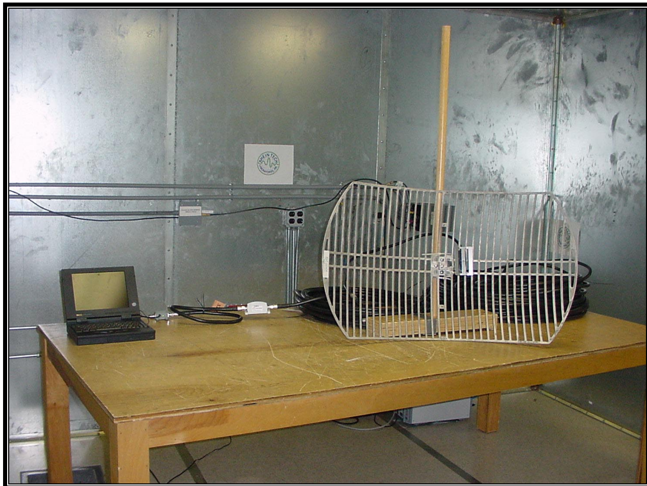
PHOTOGRAPH 4: CONDUCTED EMISSIONS FRONT VIEW WORST CASE CONFIGURATION
