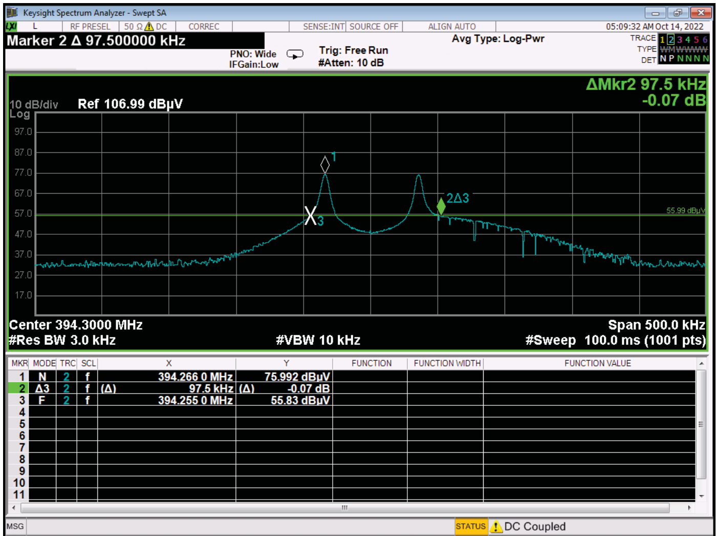
-20 dB Bandwidth Plot – High Channel
