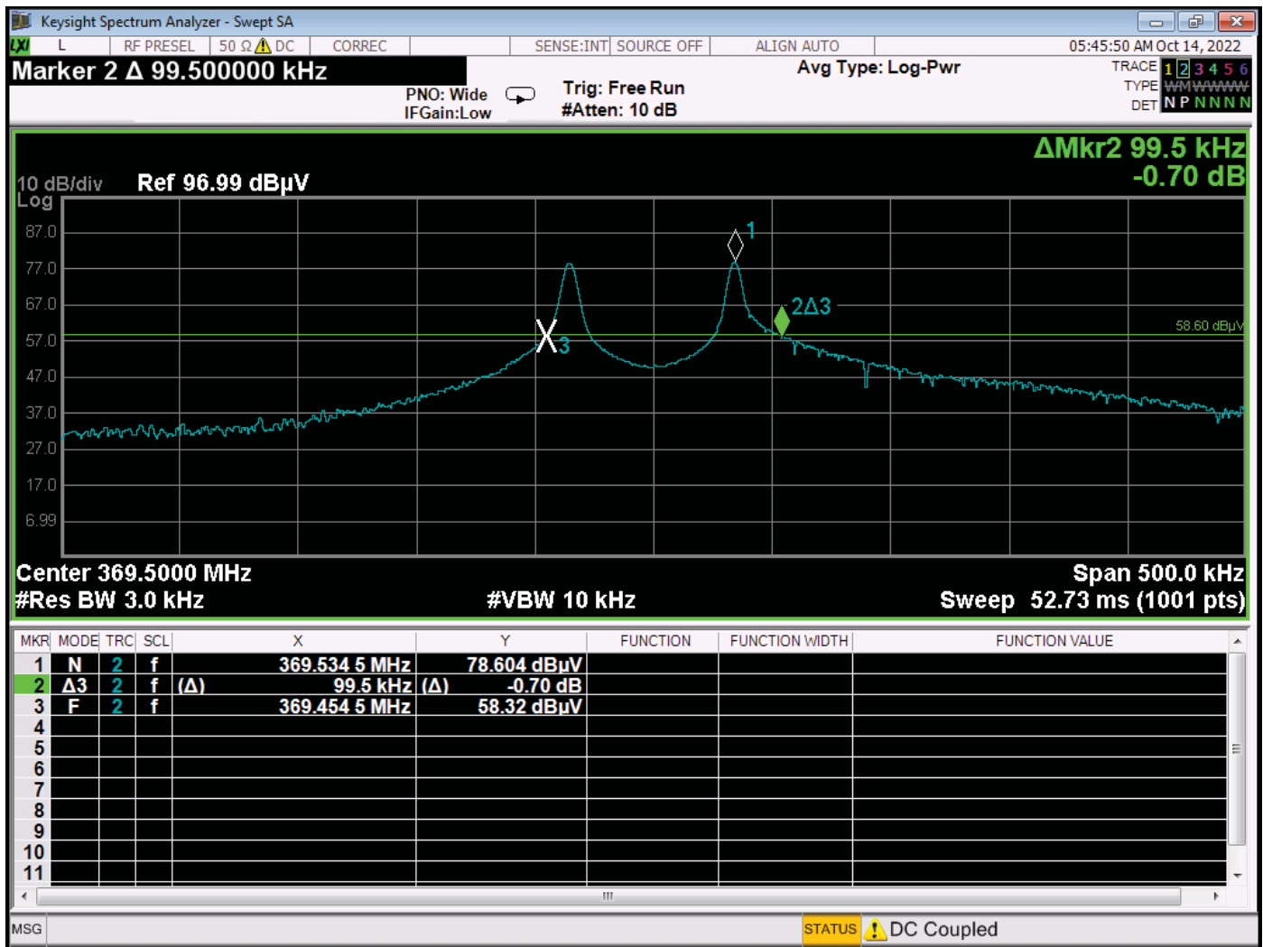
-20 dB Bandwidth Plot – Low Channel
