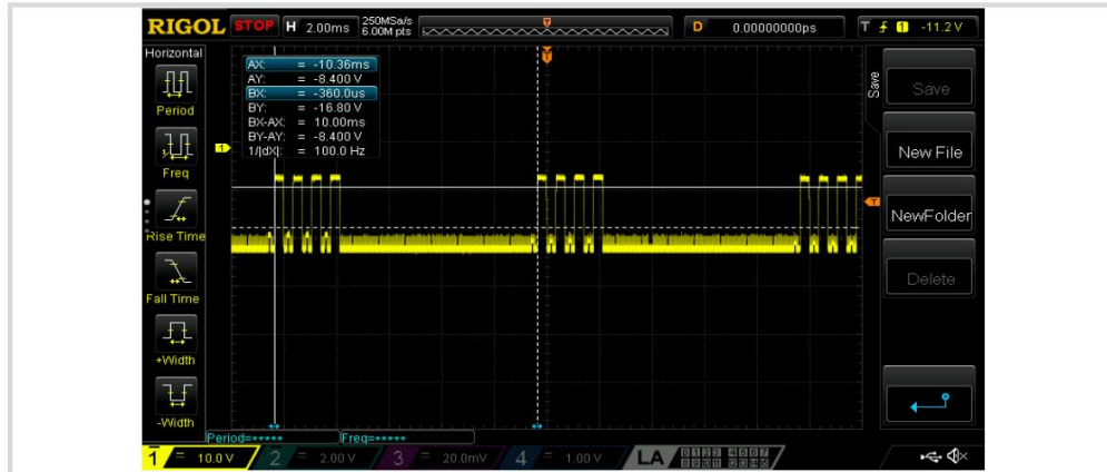
Figure 4 : Oscilloscope Graph of 10 ms Connection Interval
