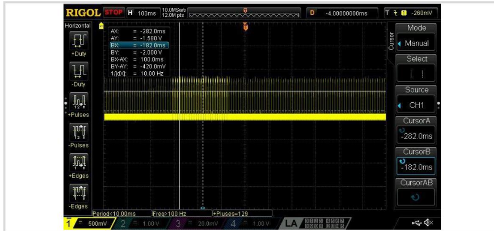
Figure 6 : Oscilloscope Graph 100 ms/div so 1,200 ms Interval
