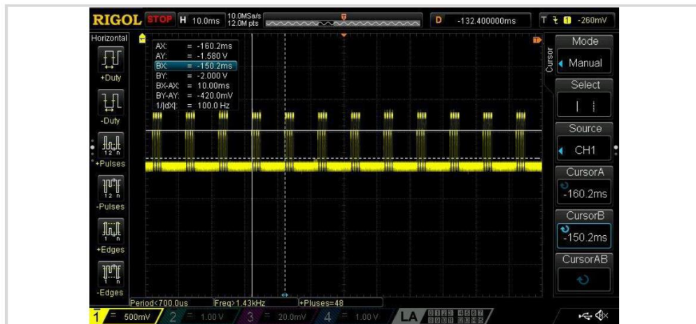
Figure 5 : Oscilloscope Graph 10 ms/div so 120 ms Interval
