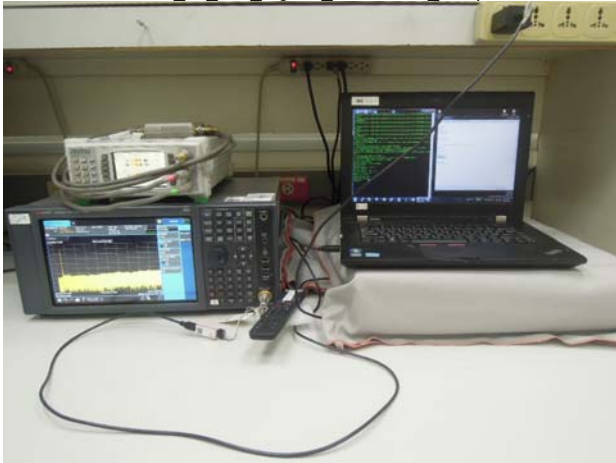
FCC 15 247 Zigbee Radiated Setup
