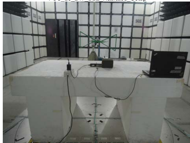
FCC 15 247 BLE Radiated Setup
