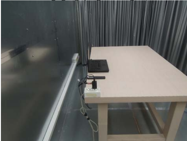
FCC 15 247 Zigbee Conduction Setup
