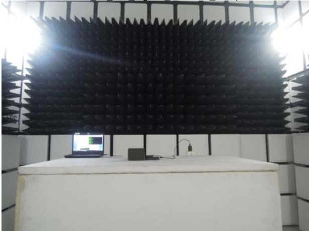
FCC 15 247 Zigbee Radiated Setup
