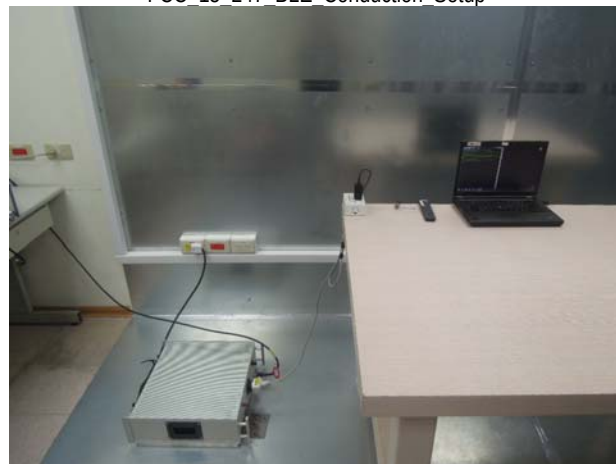
FCC 15 247 BLE Conduction Setup
