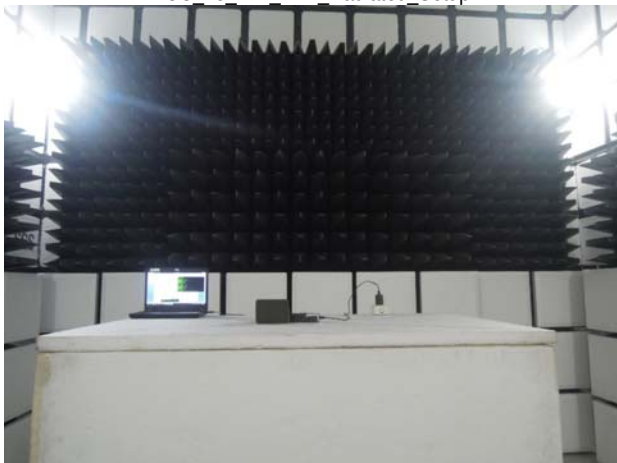
FCC 15 247 BLE Radiated Setup
