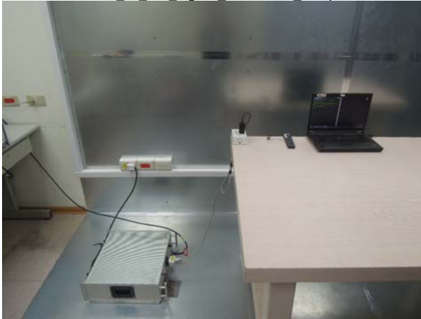
FCC 15 247 Zigbee Conduction Setup
