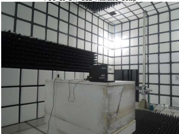
FCC 15 247 BLE Radiated Setup
