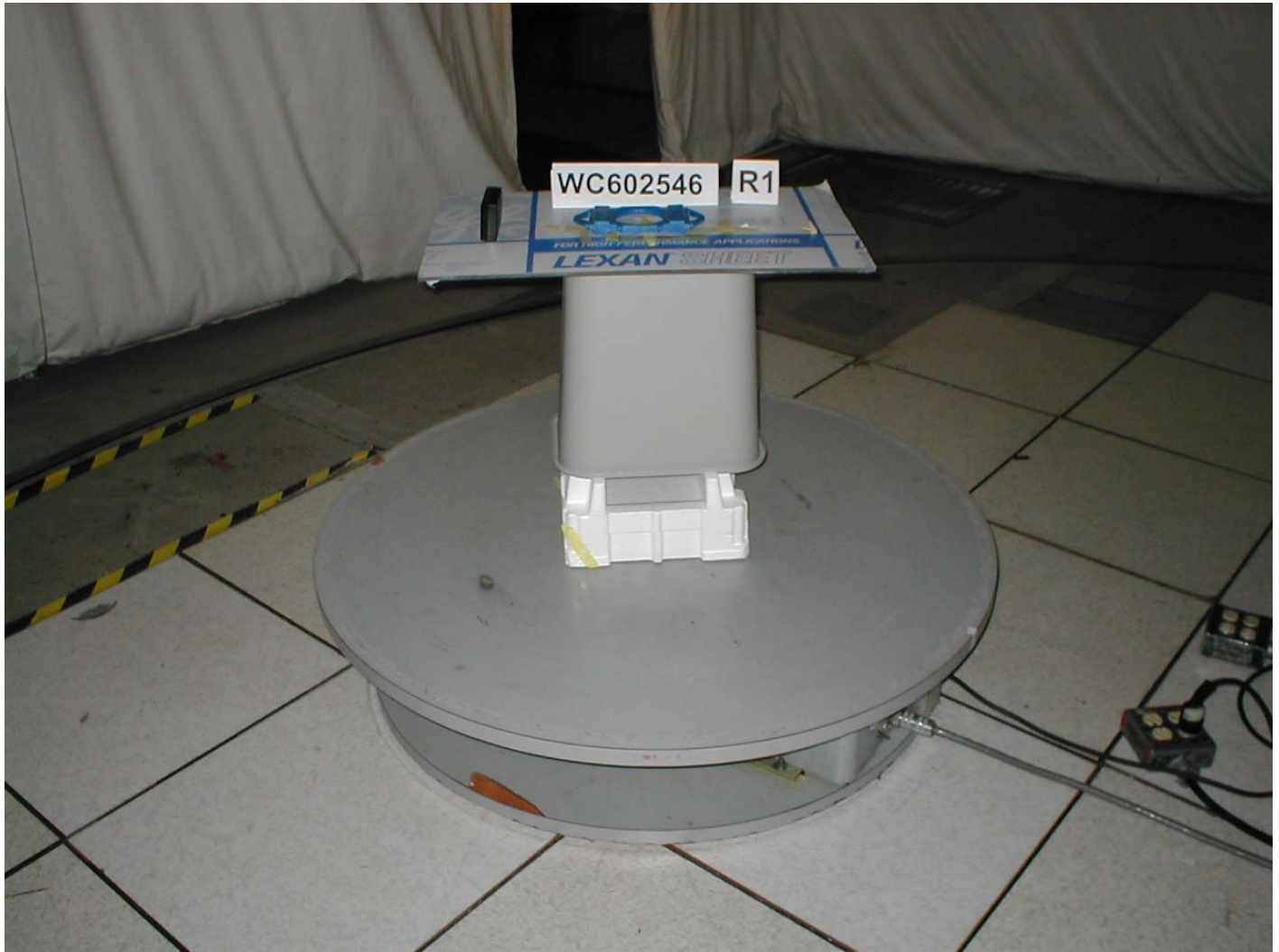
Test setup photo, radiated emissions Repeater RPT-910-3
