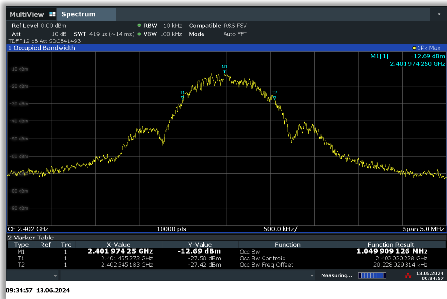
99% Occupied Bandwidth Low Channel 2.402 GHz 1M Data Rate The measured 99% OBW is 1.0499MHz
