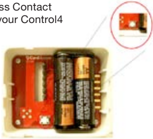
The button is located on the radio/logic board found inside the Cover Assembly.
