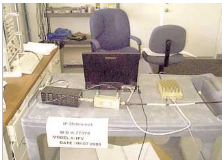
Test Setup of Bandwidth Plot Testing – Back View
