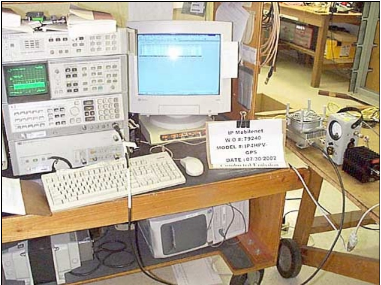
PHOTOGRAPH SHOWING CONDUCTED EMISSIONS FCC 15.111
