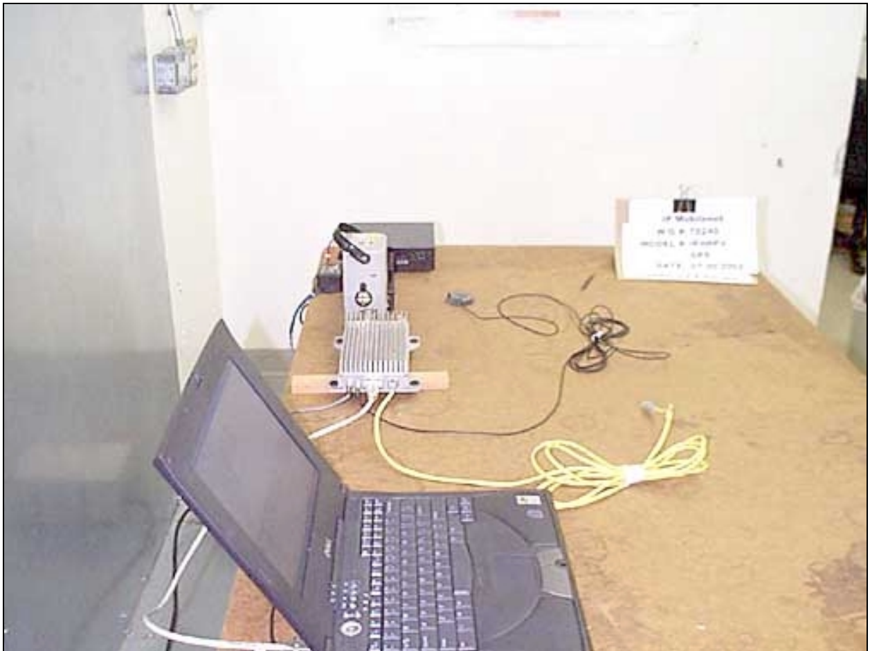
Mains Conducted Emissions - Back View - RS232
