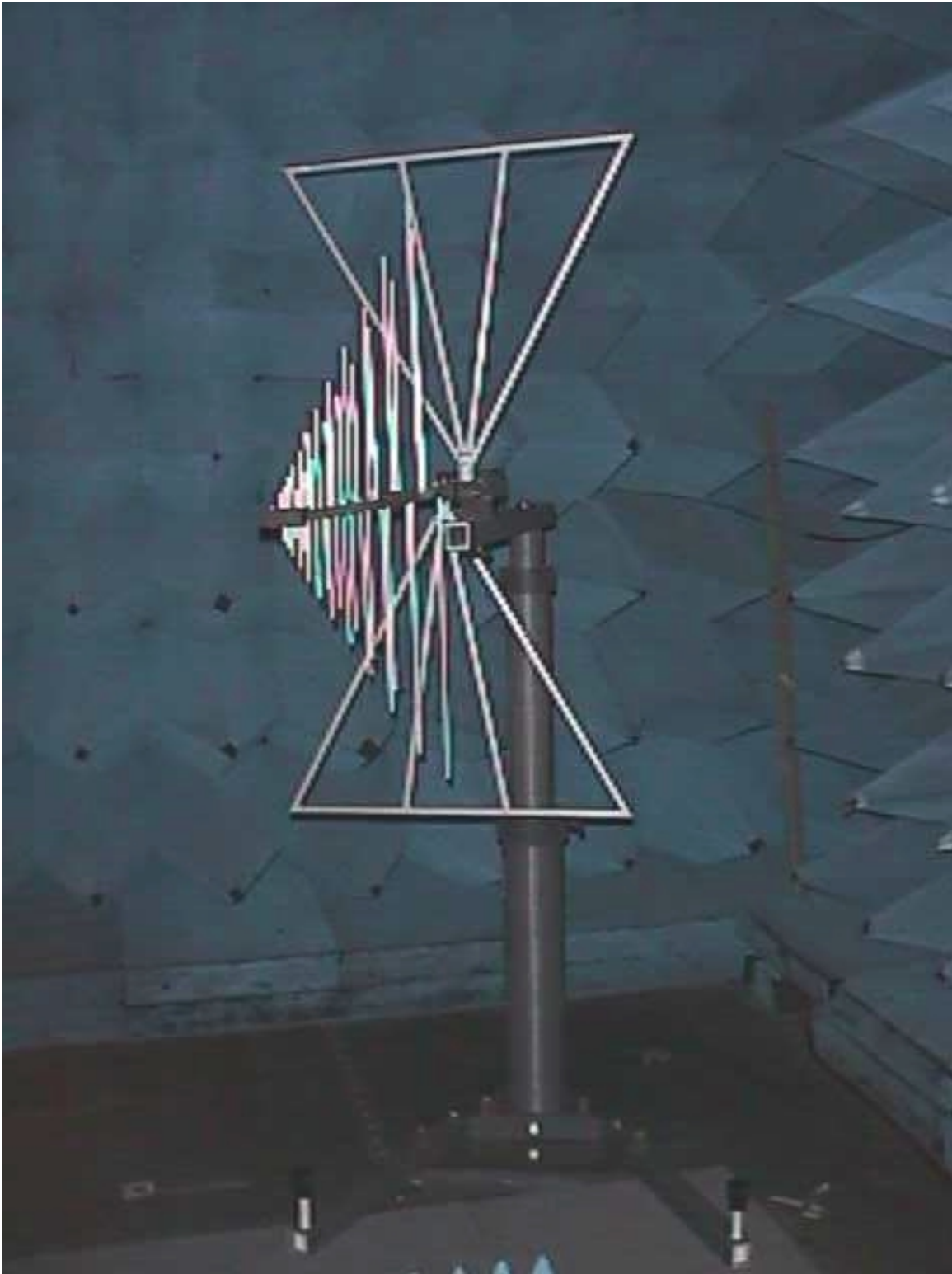
Figure B – 4 Receive Antenna, Radiated Spurious Emissions
