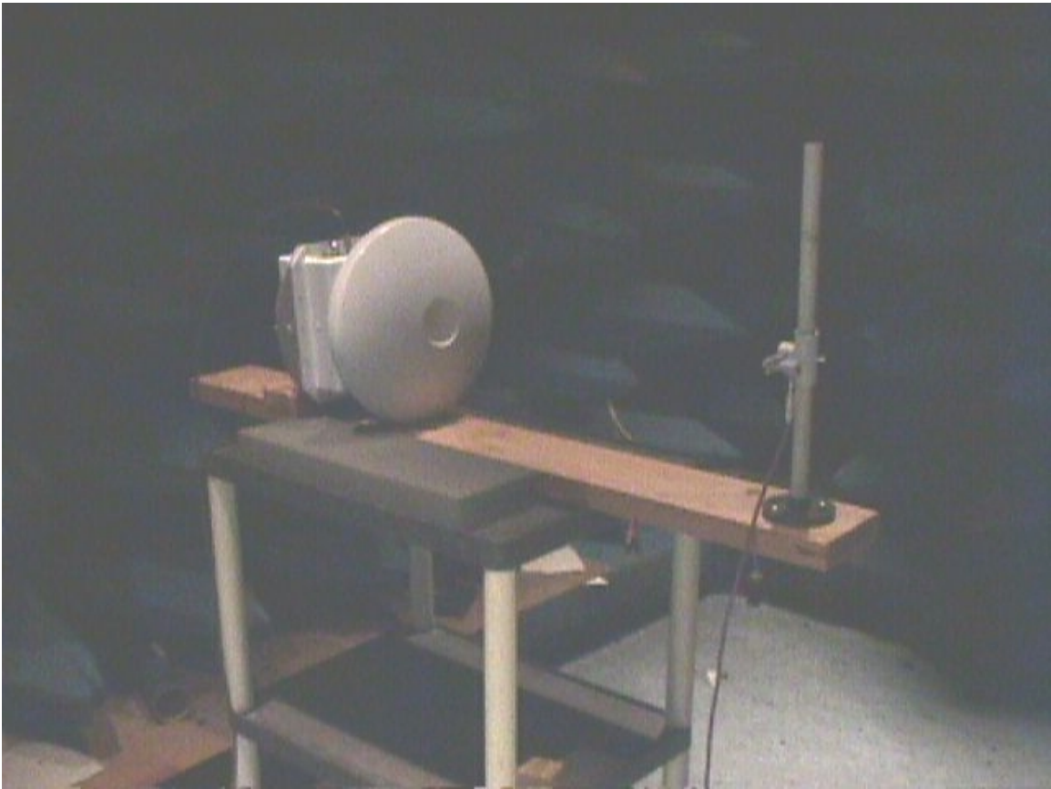
Figure B – 3 Motorola ODU Setup, Radiated Spurious Emissions
