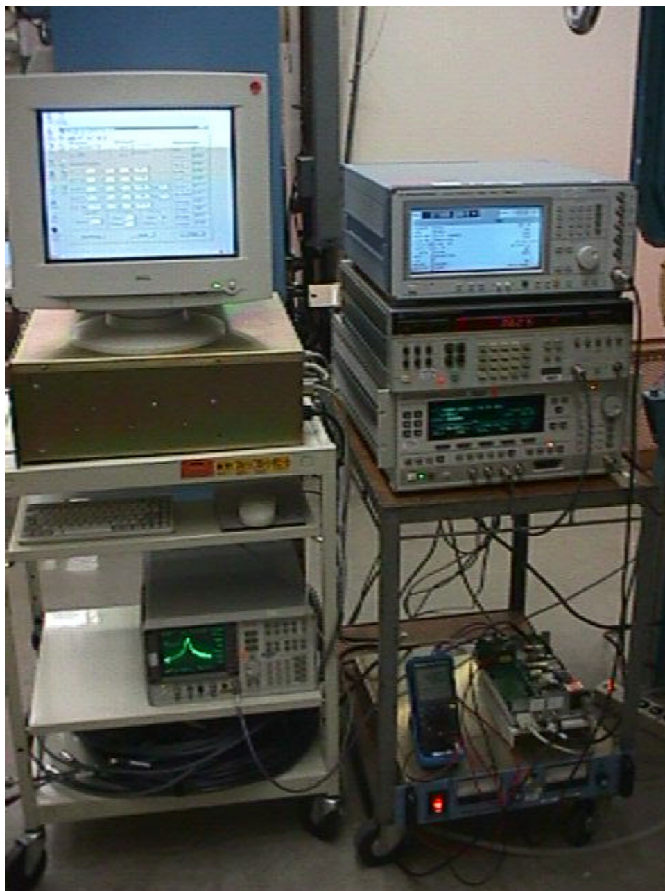
Figure D – 3 Test Setup, Frequency Stability Testing of the Zephyr ODU
