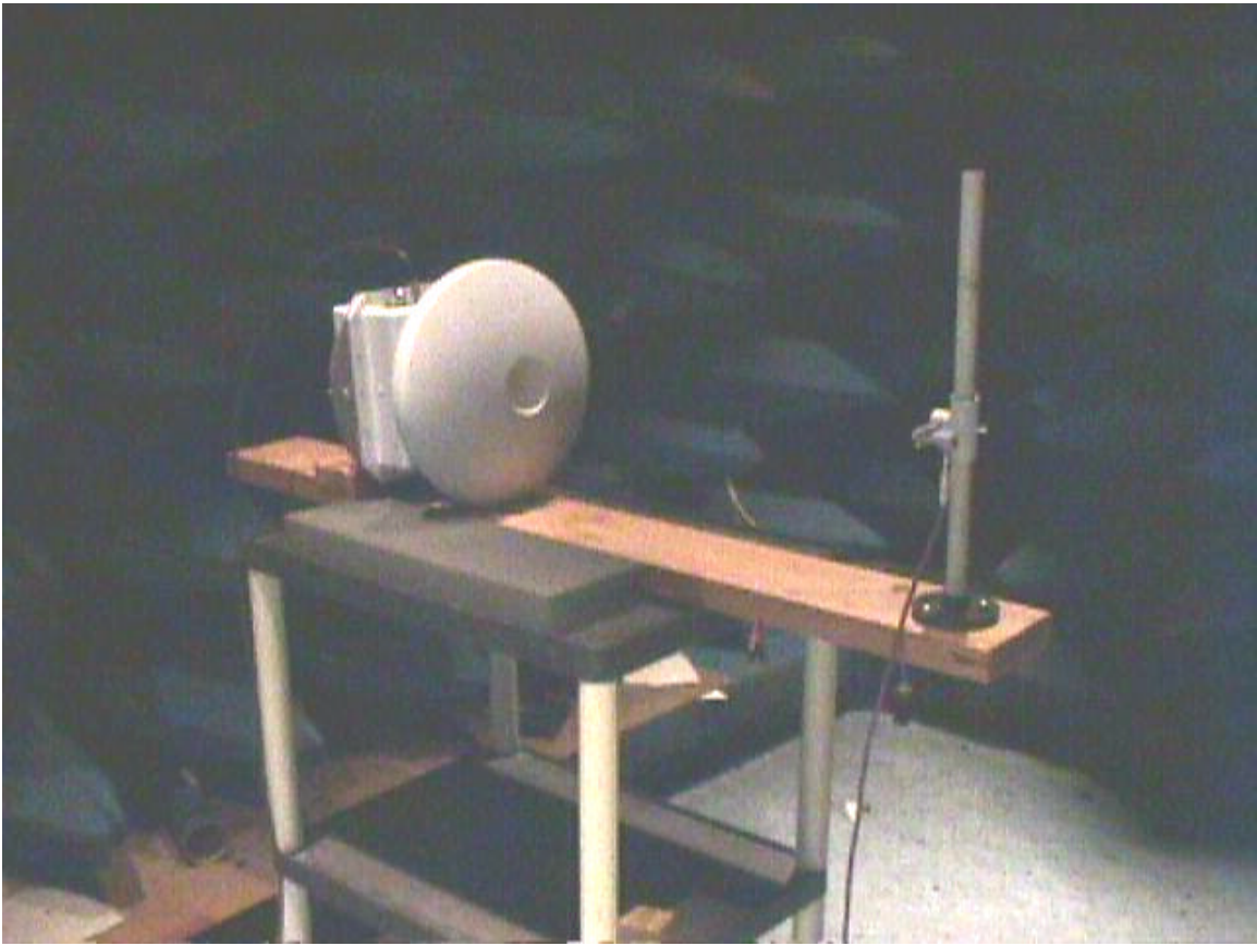
Figure C – 4 Zephyr ODU Setup, Radiated Spurious Emissions
