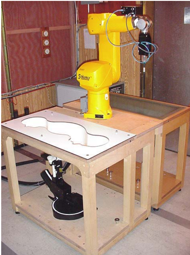
DASY4 SAR Measurement System with SAM Phantom
