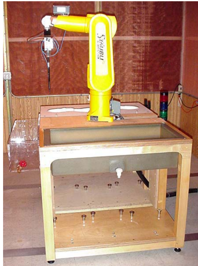
DASY4 SAR Measurement System with Planar Phantom
