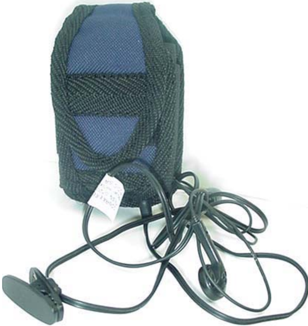
DUT with Nitelze Small Clip Case Phone Holster & Generic Earbud/Lapel Microphone
