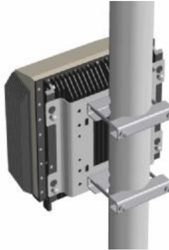
Figure 12 Insert the heads of the screws through the keyhole slots in the mounting plate and lower the TMB until the screw heads are retained by the narrow portions of the slots. (2): Tighten the screws.
