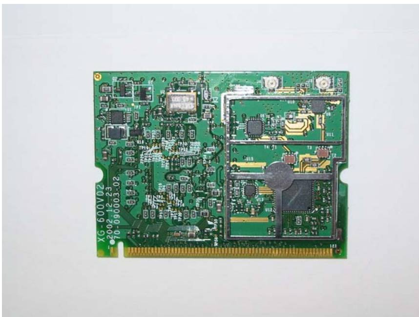
EUT – Transceiver Component with Shield Removed View
