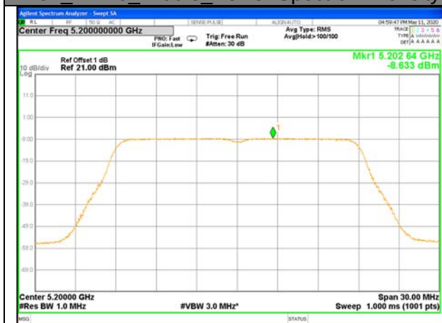
W52_11n20_Middle_Power Spectrum Density
