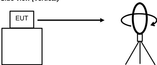
Figure 2: Direction of the Loop Antenna
