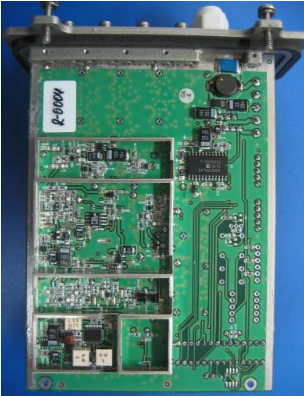
Photograph No.5 Repeater/Receiver PCB second side view without screen
