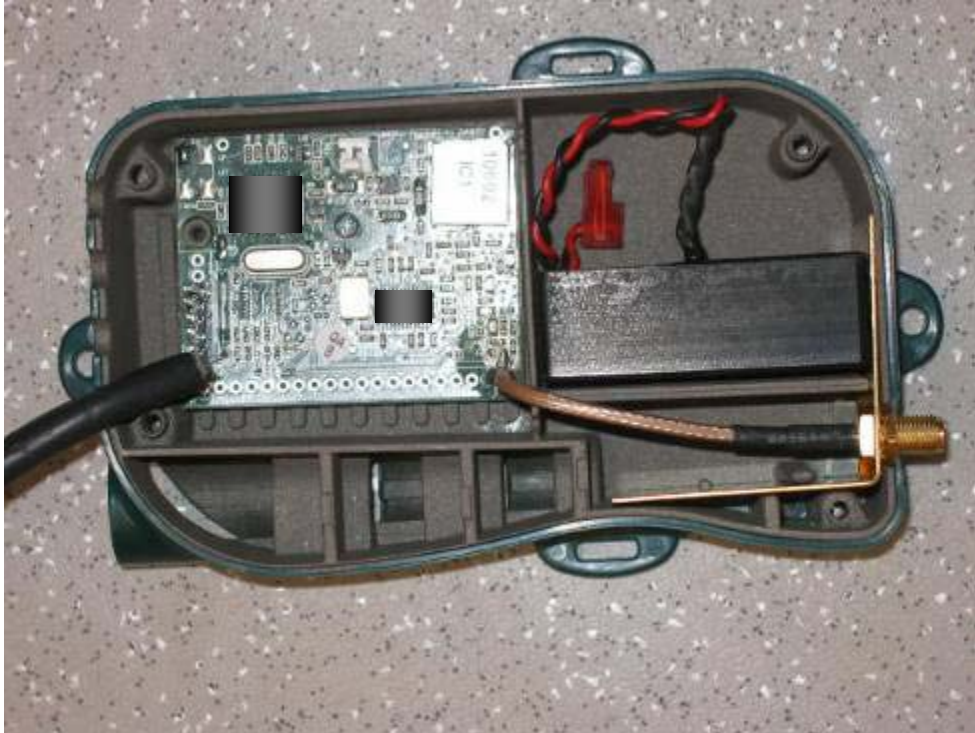
Photograph No.1 IRRIWISE-TRANS. & ANT ONE WTR METER 151 Internal view
