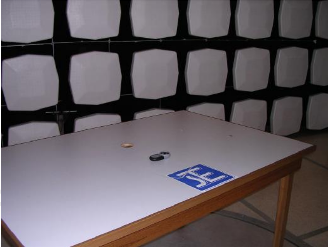
Measurement of Radiated Emission Test Set Up
