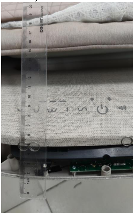
Distance between BT ANT and human body
