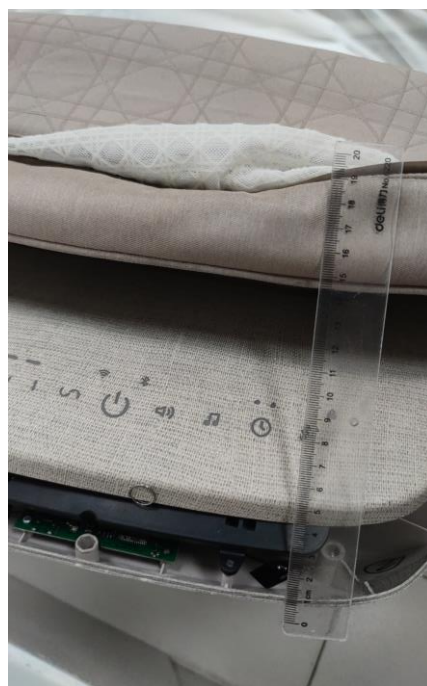
Distance between Wi-Fi ANT and human body
