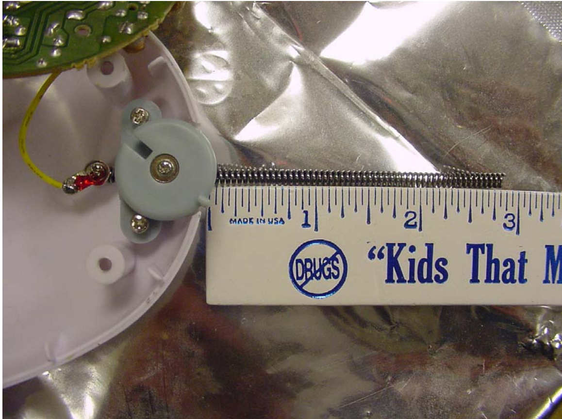
Antenna and its connection with cover removed.
