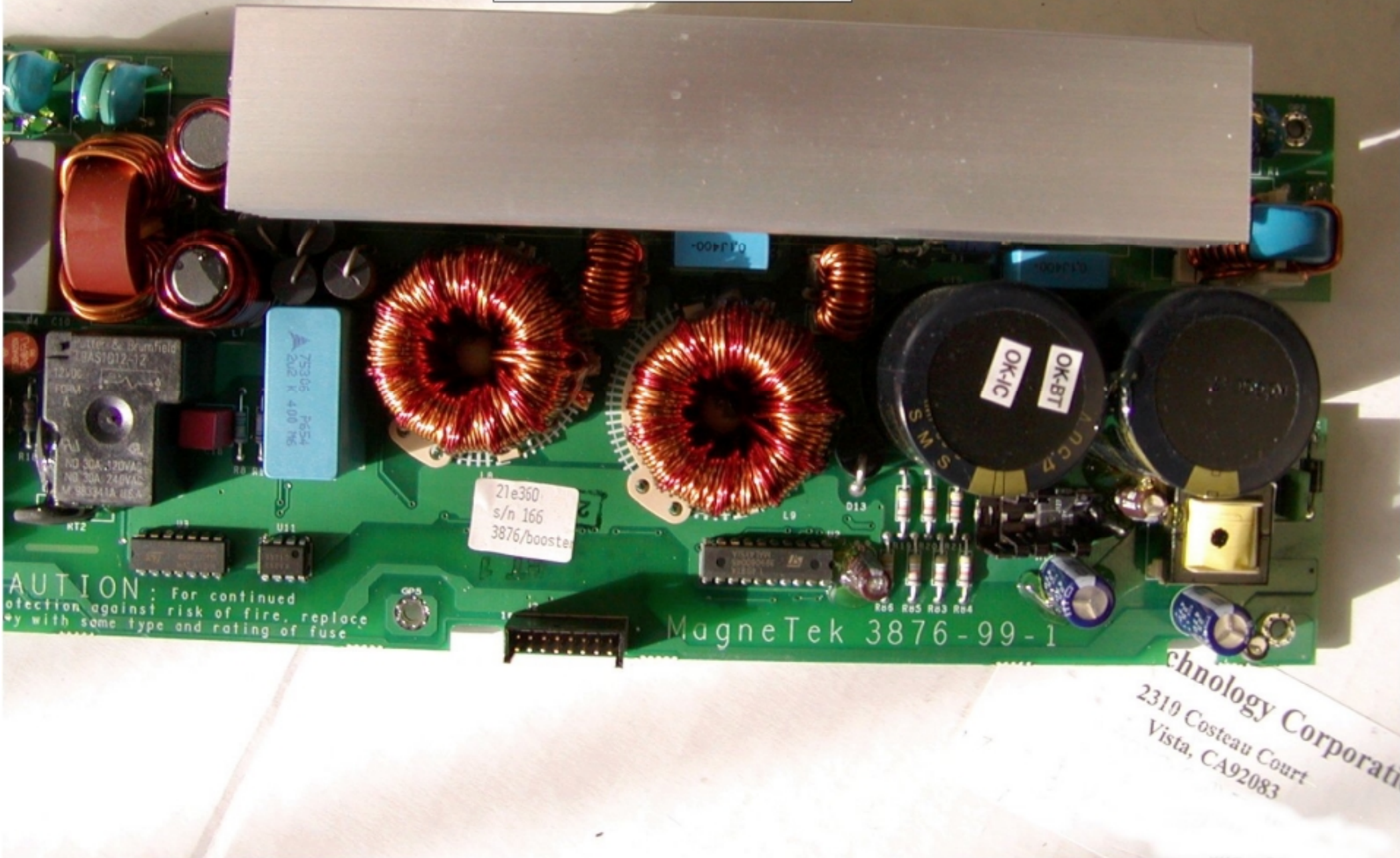
G2BT - Power Supply - Top PCB Component Side - Front
