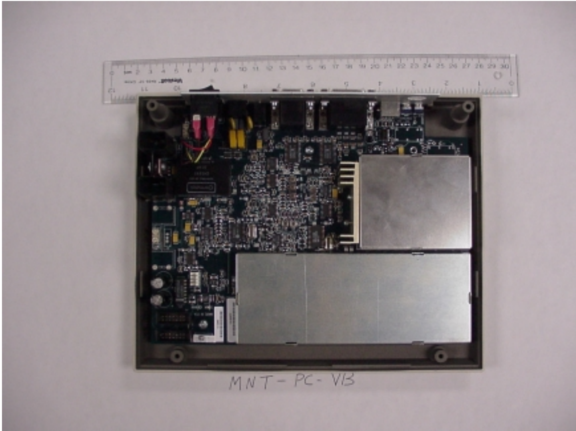
Inside, showing main board with shields
