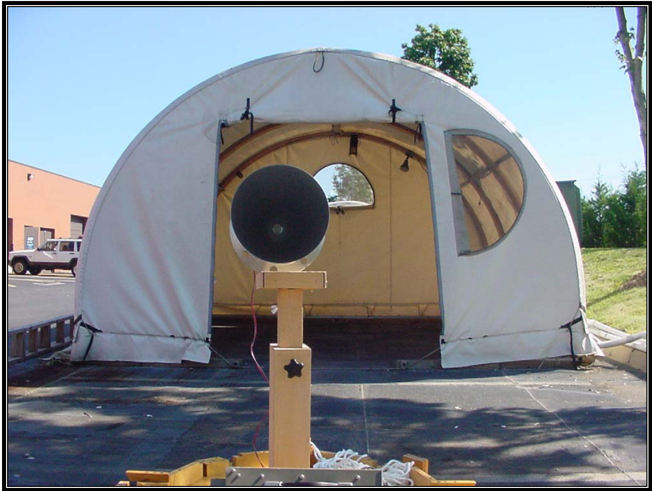
PHOTOGRAPH 6: RADIATED EMISSIONS FRONT VIEW 21.0 DBI HORN
