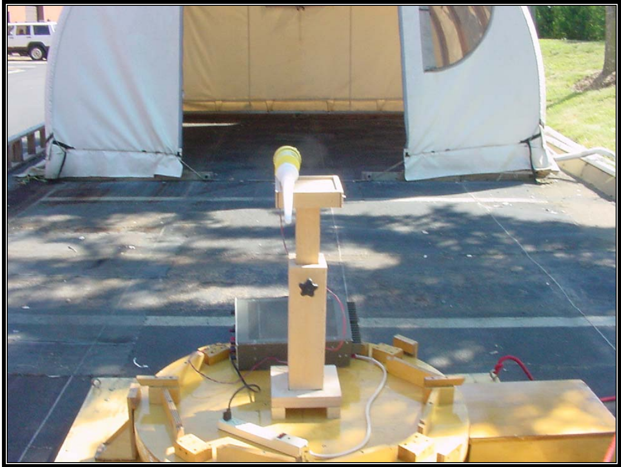
PHOTOGRAPH 2: RADIATED EMISSIONS FRONT VIEW 17DBI ROD
