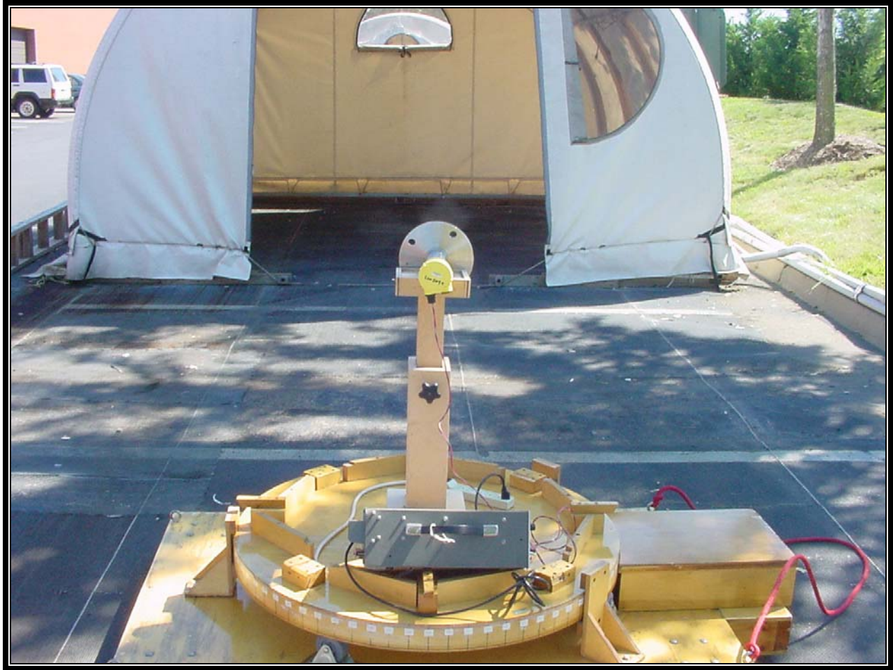
PHOTOGRAPH 5: RADIATED EMISSIONS REAR VIEW 10.0DBI HORN
