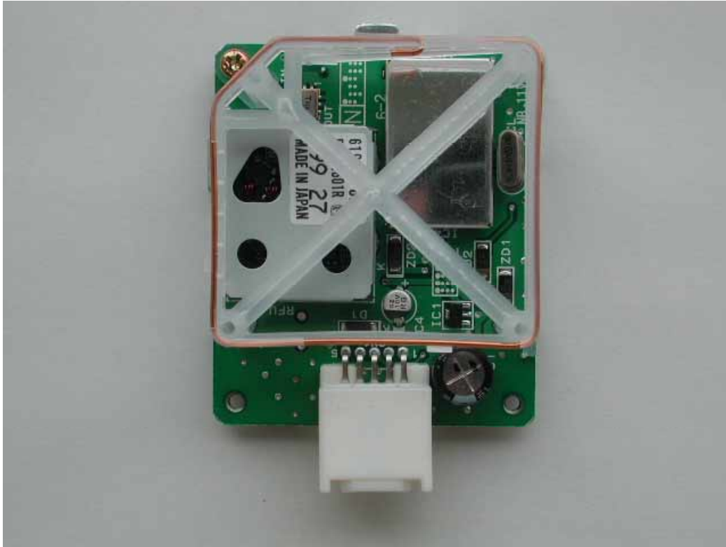
Mother PCB W/ Antenna PART No. D02PB
