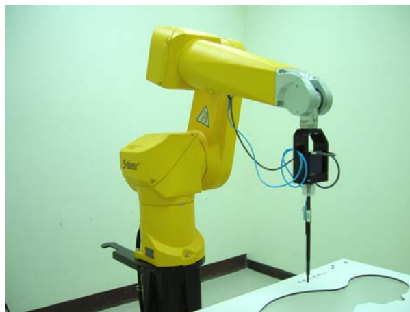
Fig. 5.2 Probe setup on robot
