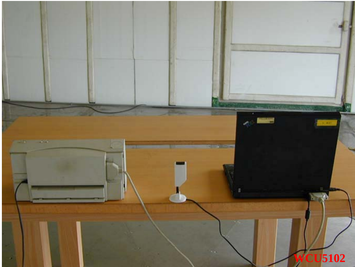
Photo 2: Radiated Emission Test Set-up
