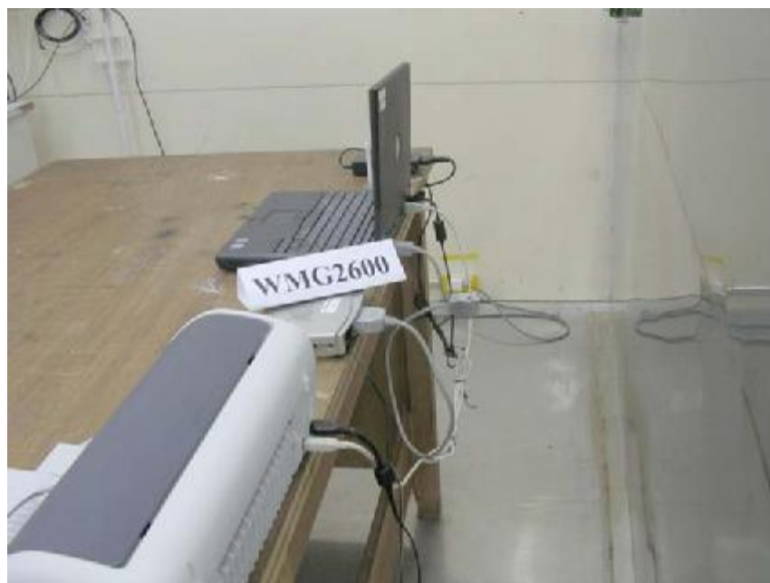
Photo 2: Conducted Emission Test Set-up
