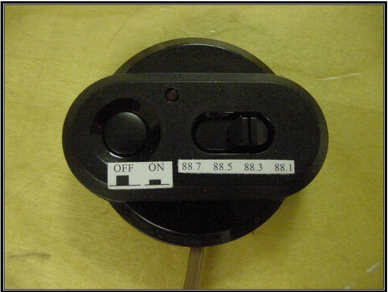
PHOTOGRAPH 6: TOP OF FM-10 Tx CONTROLLER
