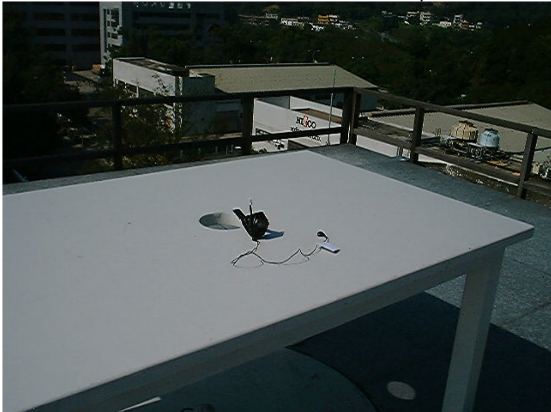
Measurement of Radiated Emission Test Set Up
