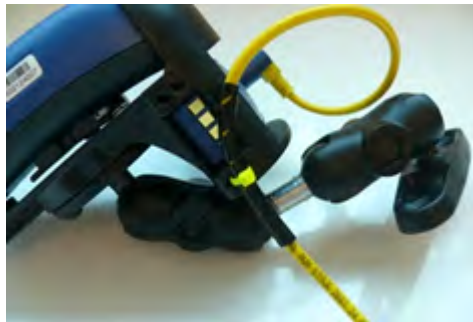
Figure 23: Cables secured on a vehicle
