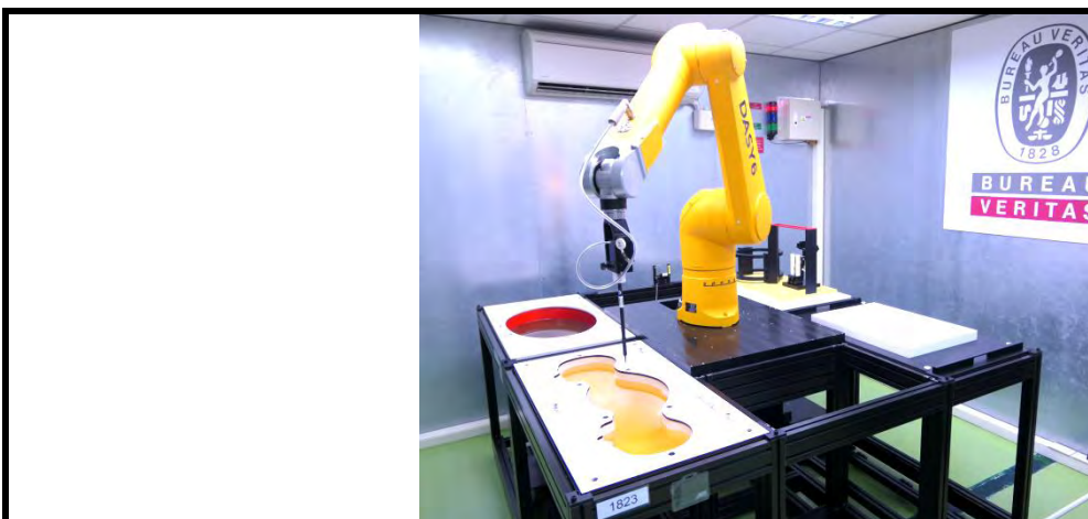
Fig-3.2 SPEAG DASY6 System
