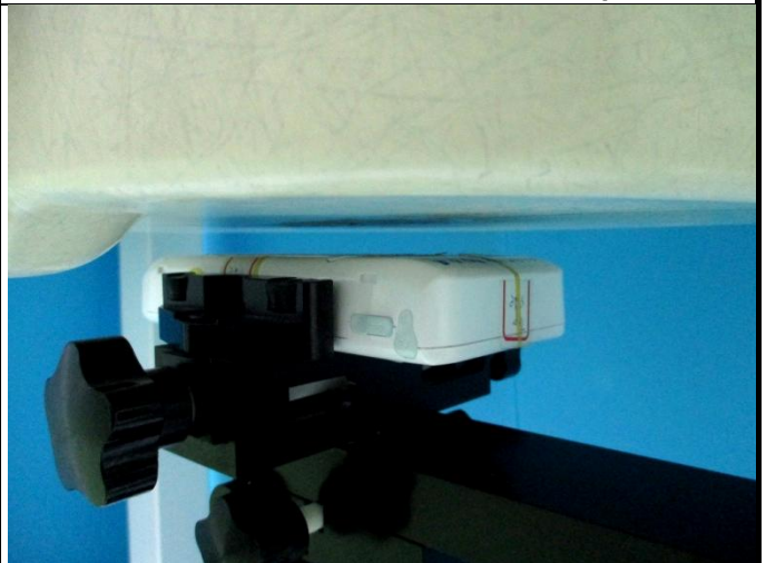
Rear Face of EUT with 1 cm Gap
