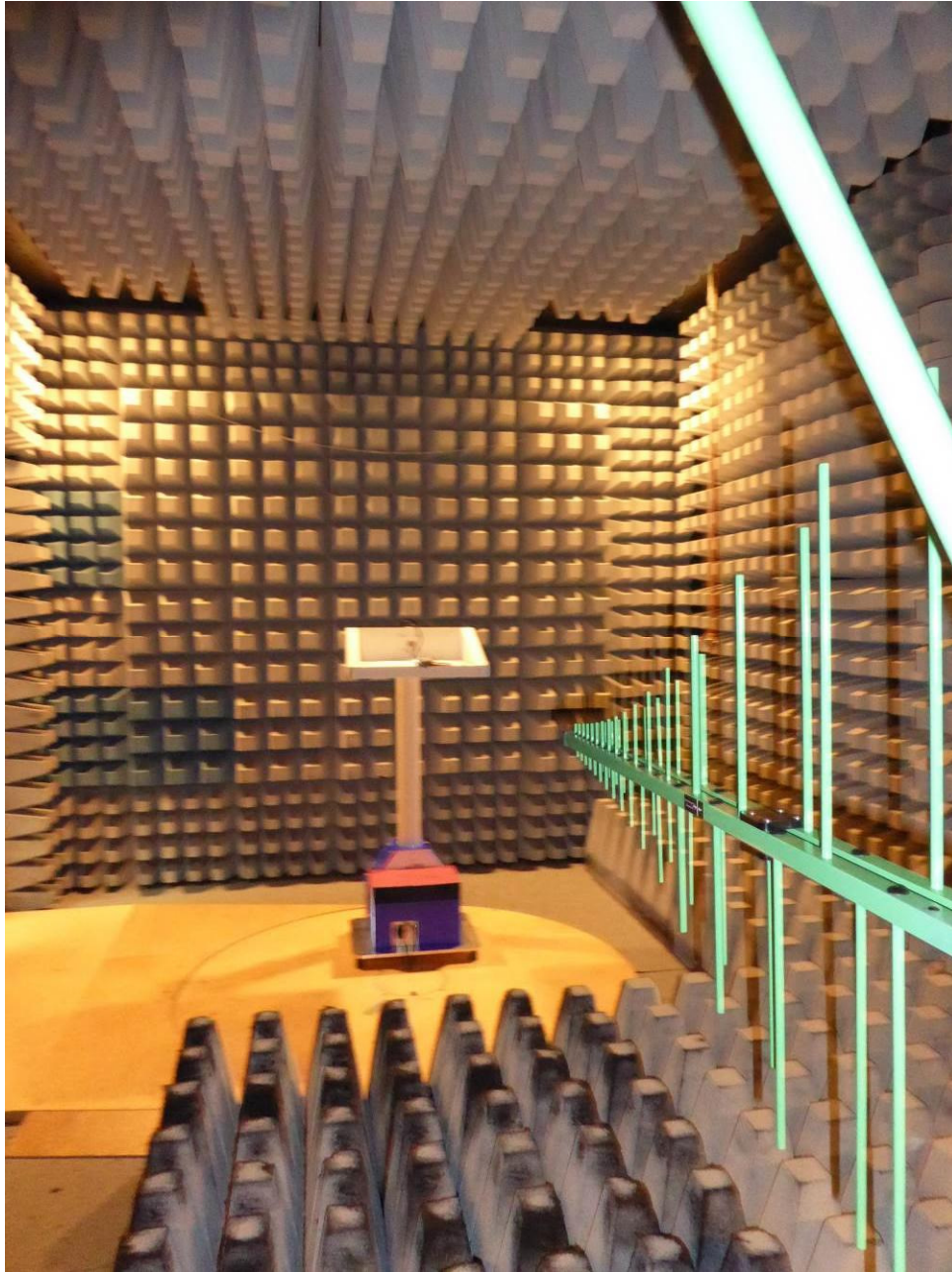
170226_06: Test setup CAH antenna - Radiated emission anechoic chamber
