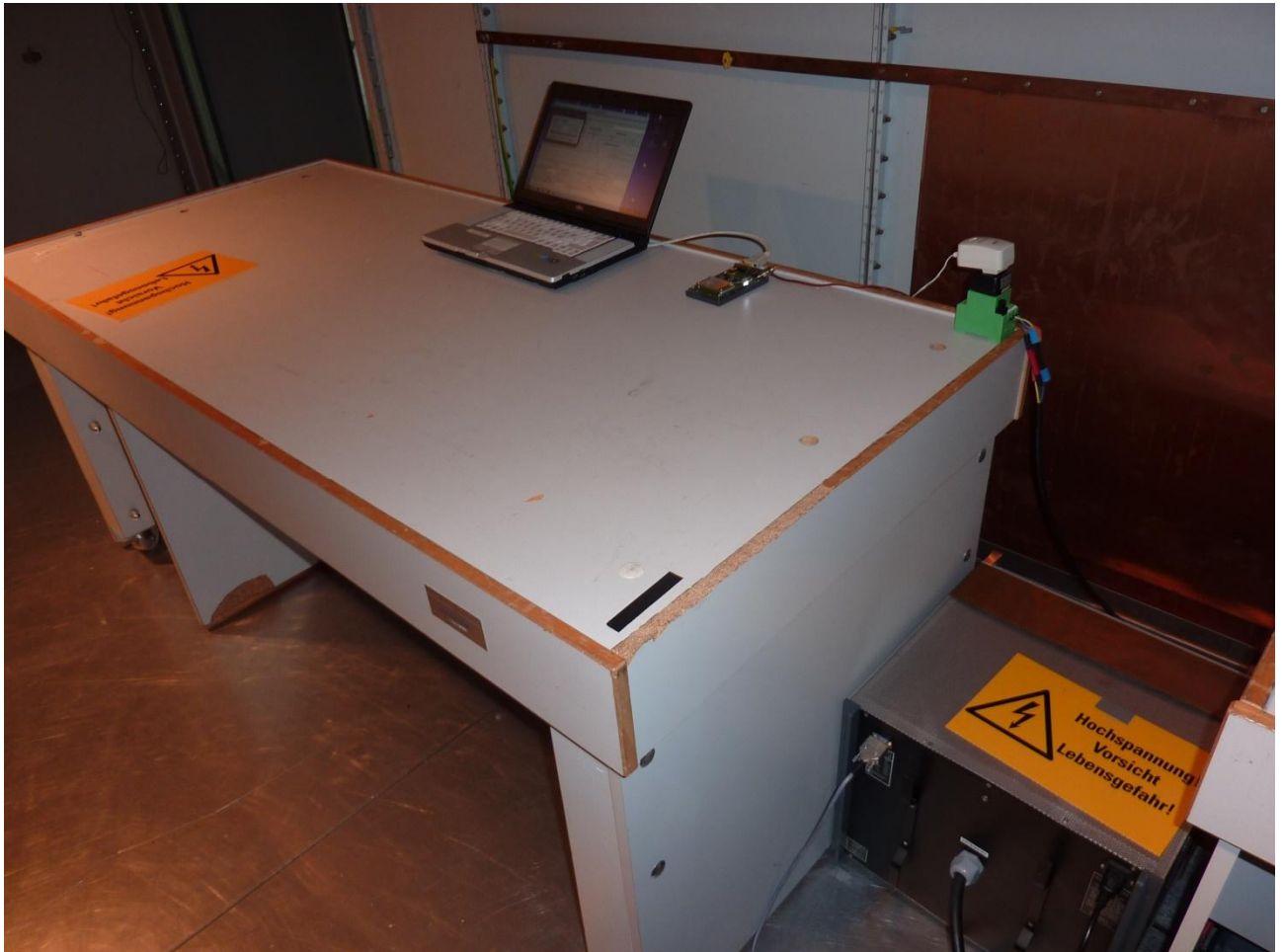
172629_16.JPG: Test setup - Conducted emissions on power supply lines
