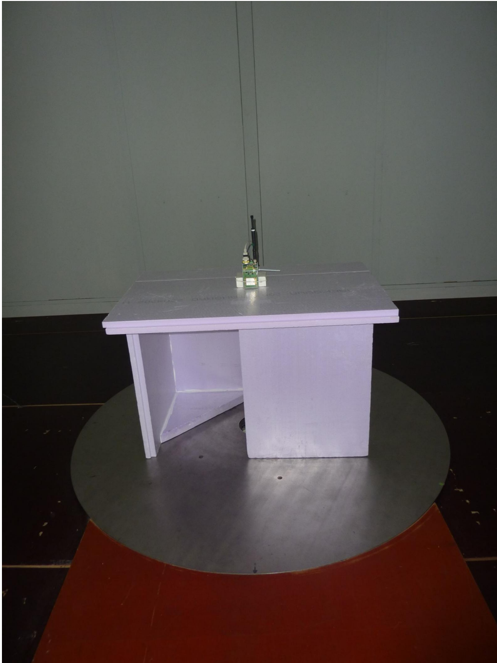
172629_22.JPG: Test setup CA915H antenna - Radiated emission (OATS)
