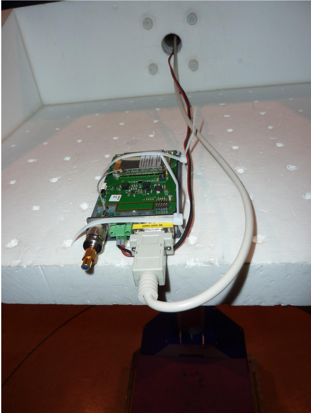
172629_19.JPG: Test setup antenna port terminated- Radiated emission (fully anechoic chamber)
